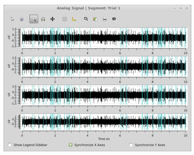
The plot shows all four signals from the first segments as well as the spike times of the inhomogeneous poisson process in the same segment.
