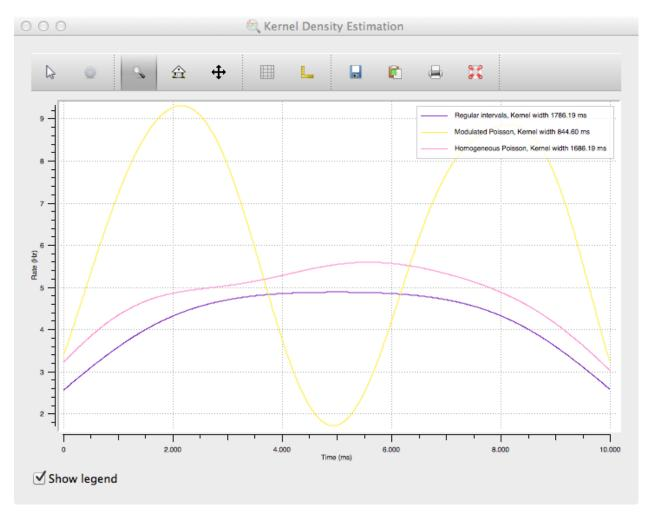
While spike density estimations are preferable to PSTHs in many cases, the picture also shows an important weakness: The estimation will generally be too low on margins. The areas where this happens become larger with kernel size, which is clearly visible from the rounded shape of the purple and pink curves (which should be flat because of the constant rate of the spike trains) with their very large kernel size.
